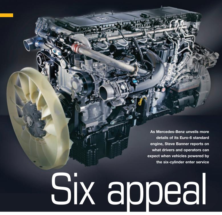
ne of the first heavy truck diesel engines to meet Euro 6 – Mercedes-Benz's new OM 471 six-cylinder in-line 12.8-litre – will be no thirstier than the manufacturer's existing Euro 5 power plants. That is the explicit promise made by Georg Weiberg, head of product engineering at Daimler Trucks in Germany.
